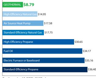
Geothermal – 4.0 COP\*, \$0.12/kwh
