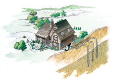
**Vertical Loops:** Used where land area is limited or soil conditions prohibit horizontal loops. Installed using a drilling rig.
